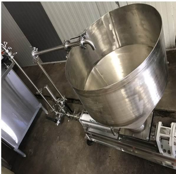
Figure 2. Specialized equipment for apple puree processing line: Apple puree processor (a), progressive cavity pump for loading equipment (b) and grinder (c).
